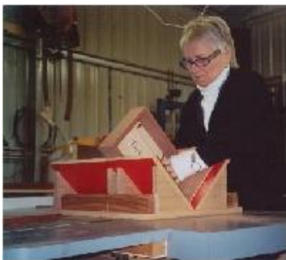
One of Tony's many jigs ..... this is to cut the splines on the corners of the box
